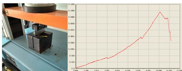
**Fig. 2:** Shear test of sweet potato seedlings
