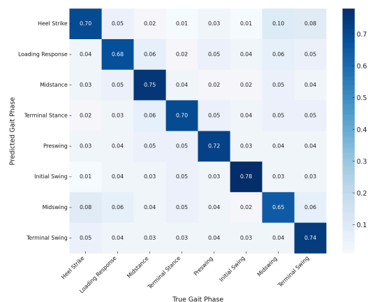
Fig. 14: Confusion matrix showing misclassification errors during validation for gait stance and swing phase classification using the PHASEY model
